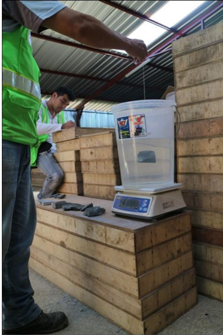
Figure 18. Water immersion density measuring procedure
