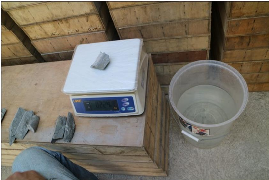
Figure 17. Density measurement electronic scales and measuring vessel
